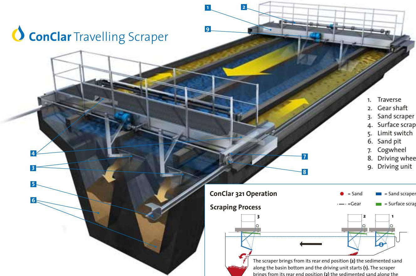
ConClar 321/325 is a travelling bridge scraper for rectangular grit chambers which can be delivered in two performances:
